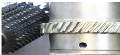
Pic.1 Hob cutter & work gear at hard hobbing
